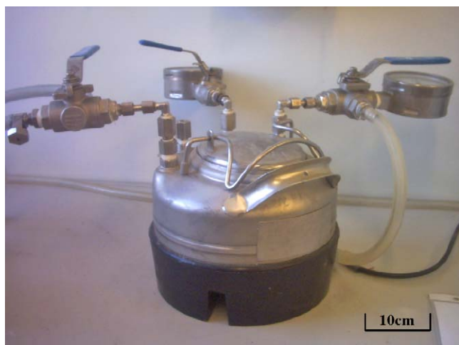
Fig. 1. Carbonation chamber equipped with a CO 2 pressure control mechanism.
